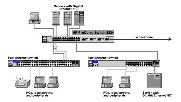
LEGEND: — Fast Ethernet cable — Gigabit Ethernet cable — Fiber cable
