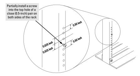
3. Place the switch in the rack and lower it so the notches in the bottom of the bracket slide onto the screws, then tighten these screws.
