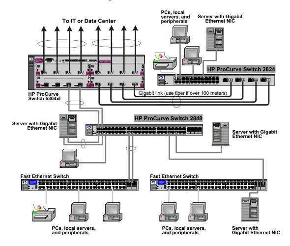
LEGEND: — Fast Ethernet cable — Gigabit Ethernet cable — Fiber cable
