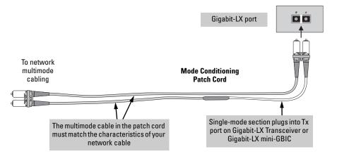
Make sure you purchase a patch cord that has LC connectors on the end that connects to the Gigabit-LX mini-GBIC, and has multimode fibers that match the characteristics of the multimode fiber in your network.
