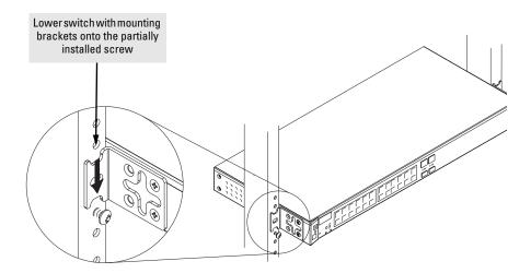
4. Install the other number 12-24 screw into the upper hole in each bracket. Tighten these screws.
