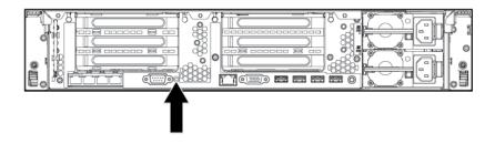
The NEBS cage must replace the commercial PCIe riser cage. Locate the visible gaskets under the PCIe riser cage blanks to identify the NEBS cage. There are no gaskets installed on the commercial PCIe riser cage. To replace the PCIe riser cage:
